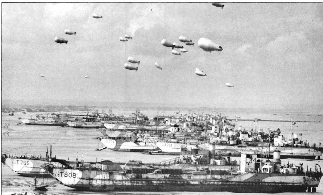
Left: LCTs "dry out" along the Normandy coast. Every landing craft was fitted with a barrage balloon which protected the vessels from low-flying German aircraft. Below: As the troops push their way inland, Coast Guard landing craft land reinforcements on the Utah beaches.
