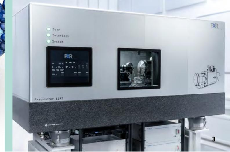
2 3D analysis with microscopic resolution: One application, as shown here, is to perform quality control and failure analysis on lithium electrodes for battery research with a voxel sampling of 140 nanometers.
