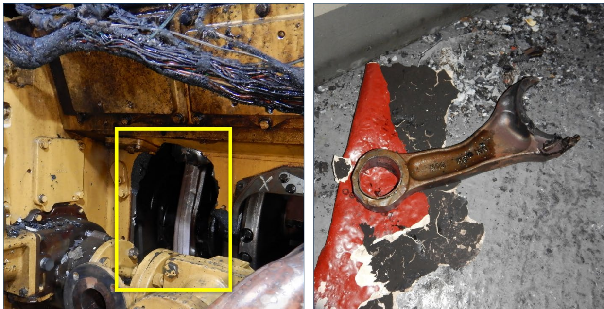
Figure 3. The damaged section of the engine ( left ), as indicated by the yellow square, from where the connecting rod from the no. 3 DG ( right ) was ejected. (Source: Oceaneering International, Inc.; Coast Guard)
