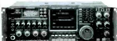
**Multi-Function Five Inch CRT.** Displays frequencies, modes, memory contents, operating notes, RIT, two menu screens, plus a panoramic view of all signals in a selected range. A portion of the screen also serves as a display for data modes like RTTY, AMTOR, and PACKET.
