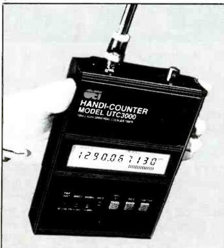
MODEL UTC-3000 is used to measure frequencies, periods, time intervals and ratios of frequencies. Applications include the identification of broadcast frequencies at maximum distance from the source; test and calibration of transmitter frequencies, medical equipment, oscillators and other types of electronic gear. It locates noise sources, serves as signal strength indicator and satisfies hobby interests as well.
