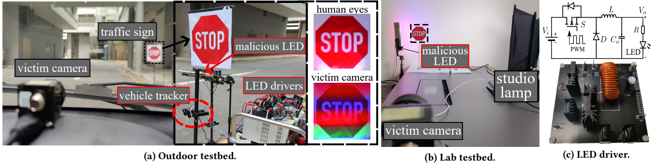
Figure 8: Testbed setups and the LED driver.
