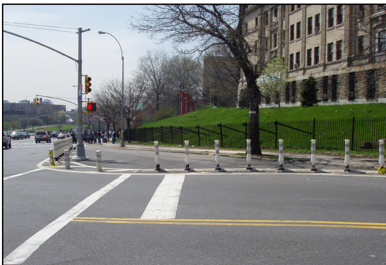
Detailed views of additional pedestrian space created by the use of curb mounted delineators and markings
