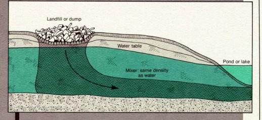
taminants which affects how they move in the ground. Gasoline, for example, is lighter than water and so floats on the top of the water table, just as it floats on the top of a lake. Therefore, gasoline is difficult to detect since it may not appear in water being drawn by a well until the water table drops to the level at which the water is being drawn. Based on their density, contaminants are sometimes characterized as "floaters," "mixers," or "sinkers."
