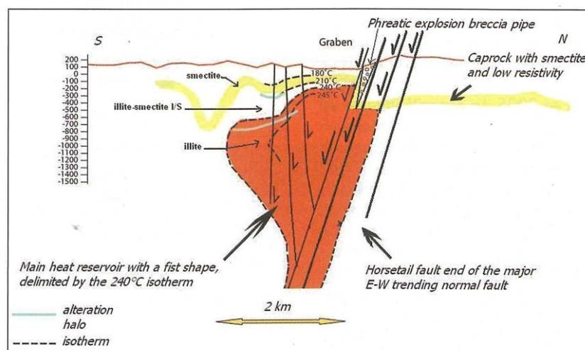
Figure 7: 2D conceptual model of Bouillante geothermal field (From Bouchot et al., 2010).
