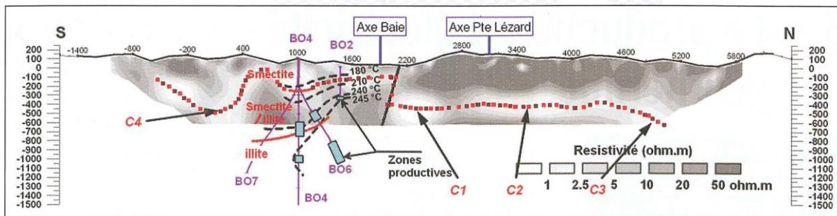
Figure 6: Isotherms and hydrothermal alterations horizons deduced from wells and the interpreted electrical profile across Bouillante Field (8 km N-S). (From Bouchot et al., 2010).
