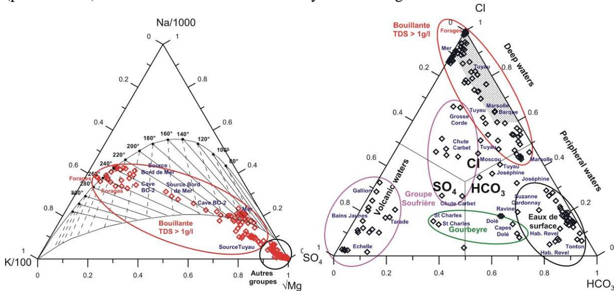
Figure 4: Na-K-Mg and Cl-SO<sub>4</sub>-HCO<sub>3</sub> ternary diagrams (Giggenbach, 1988) applied to thermal waters from Bouillante and Basse-Terre.
