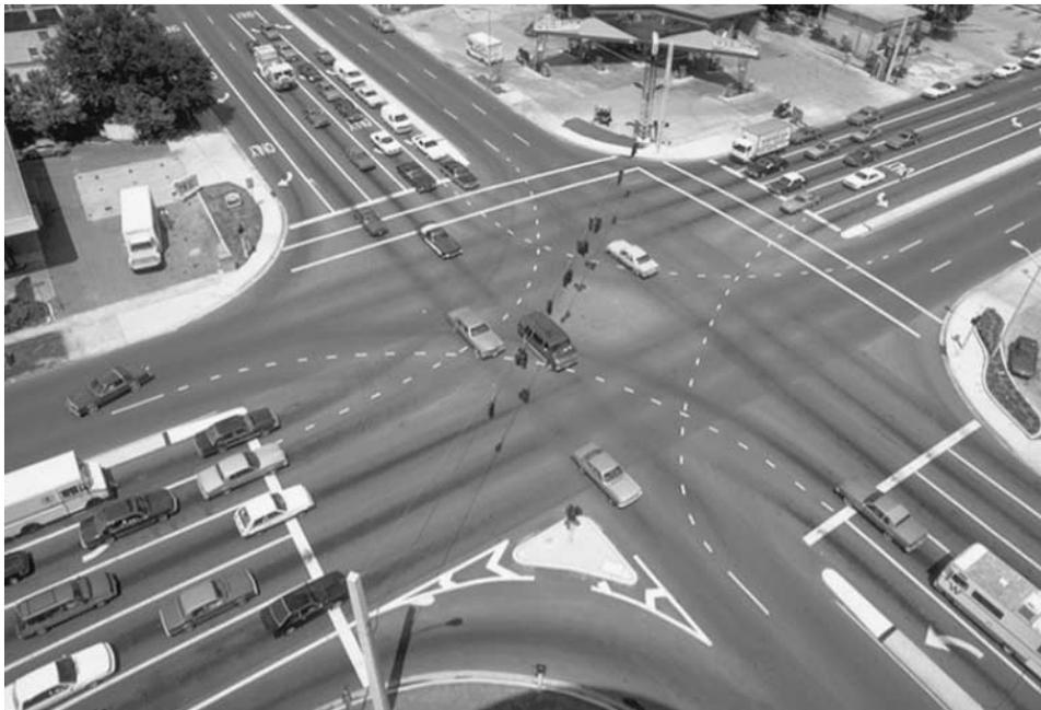
turning right for which a clear path is not readily apparent. This strategy is also appropriate for application where the roadway alignment may be confusing or unusual, such as a deviation in the path for through vehicles. Providing positive guidance to the driver in the form of pavement markings can help eliminate driver confusion and eliminate vehicle conflict by “channeling” vehicles in their proper path.
