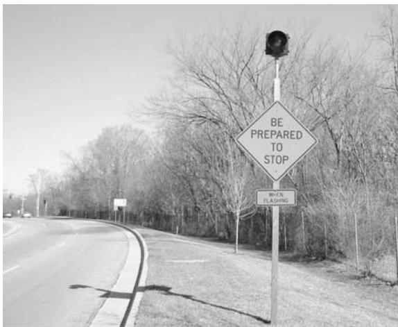
Providing a break in pavement markings at intersections also helps to alert drivers to their presence. This includes centerlines, lane lines, and edge lines. Close spacing of progressive signals can lead to drivers focusing on a downstream signal and not noticing an intermediate signal. Signing, pavement markings, lighting, or alteration of the appearance of a signal to make it more noticeable should be considered in this situation.
